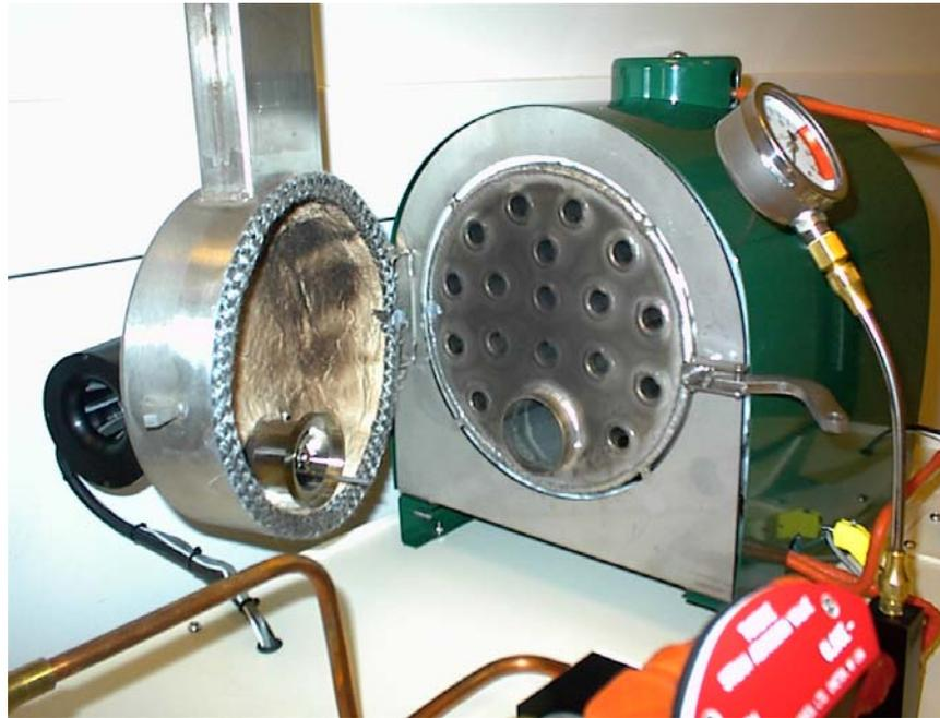
**Fig. 3:** The boiler (open). The flame burns in the large pipe, and the hot combustion gas returns through the smaller pipes to the exhaust chimney. The burner is mounted in the door. The lower part of the boiler contains liquid, the upper part contains steam. At least the upper five pipes are surrounded by steam, which can be superheated.
