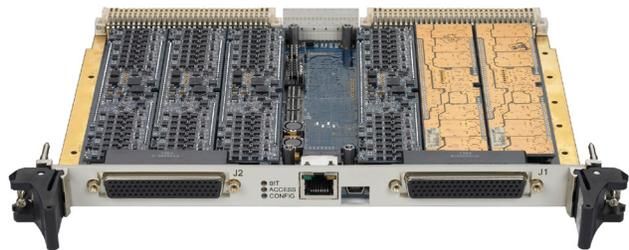
In addition, if the inputs and the outputs of a synchro are not *galvanically isolated* from each other (and from the signal ground) common mode noise can dramatically affect the accuracy of conversion. To avoid these problems, an S/D converter board must employ transformer-isolated inputs and outputs, thus significantly reducing the effects of common mode noise and ground loops.
